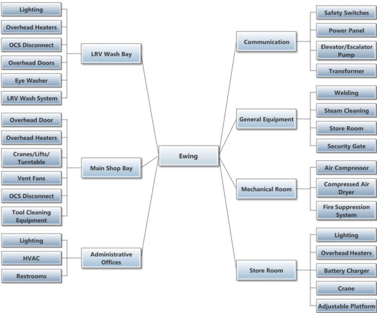
Figure 4-7 Typical Rail Maintenance Facility Hierarchical Components
